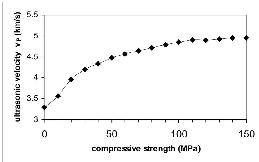
Fig. 9 Ultrasonic velocity  $v_p$  of greywacke cylindrical samples vs. compressive strength.
